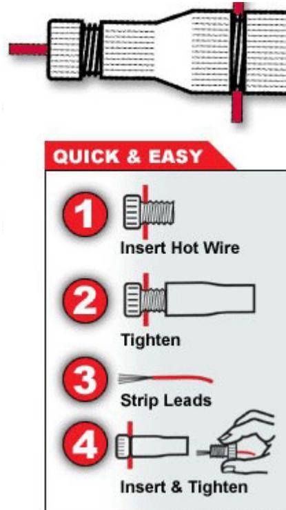
**Scheme 4. How to connect the wires using Posi-Taps.**
