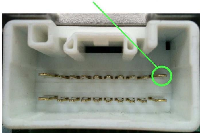
**Picture 3: Constant POWER wire location on the main vehicle harness**
